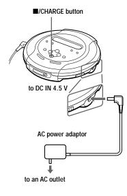
The CD player charges the batteries. The "Charging" indicator turns on in the display, and the indicator sections of [III] light up in succession. When the batteries are completely charged, the "Charging" and [III] indicators turn off. If you press [III]/CHARGE after the charge has already been completed, the [III] indicator flashes and "FULL" appears in the display.
